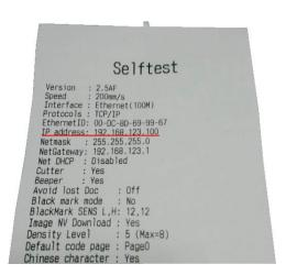
2.Confirm the printer IP address and then connect the printer to a computer through a hub, switch or cable directly (direct interconnection method). (Note: the IP address may not be modified if the connection is established through a router) Change the IP address by the test tool software in the CD, the software is as follows:
